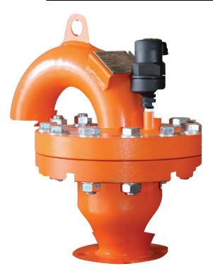
**DUAL**'s Air/Vacuum Release and Vacuum Breaker's function is to automatically exhaust large volumes of air from the system when it is being filled and also to allow air to re-enter the pipe line when being emptied. The orifice size is generally the same size as the valve inlet and outlet.
