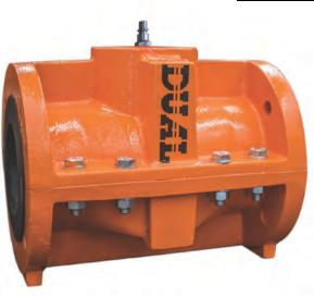
**DUAL**'s Pneumatic Valve consists of a tough, but flexible full bore sleeve in an enclosed body. Actuated by means of air or Hydraulic Fluid, the valve body acts as an Actuator. When the media is introduced,
