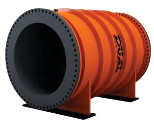
flexible full bore sleeve in an enclosed body. Actuated by means of air or Hydraulic Fluid, the valve body acts as an Actuator. When the media is introduced, the sleeve is compressed forming a complete and effective seal.
